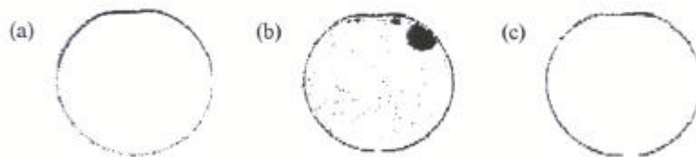
Figure 4. SAM images of bond-annealed Si-Si prepared using an SC-1 last clean: (a) unimplanted device; (b) 5e^{15}/\text{cm}^2 P implant; (c) 5e^{15}/\text{cm}^2 P implant with surface anneal.
