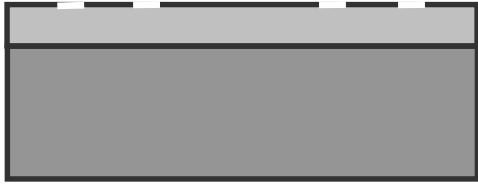
1. Oxidise Standard SOI and RIE Pattern
