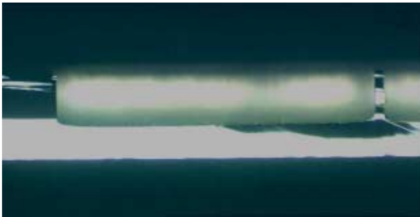
Figure 19: High exposed Area Through the Handle DRIE Process - 350 \mu m Deep into a 600 \mu m Wafer.
