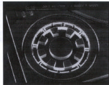
Fig. 2. SEM image of micromechanical gyro, made by Deep RIE on a bonded SOI substrate (© Crown Copyright, DERA, 1997).
