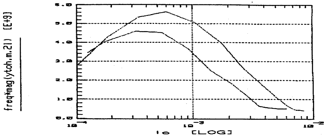
Figure 5. f_T plot of 0.75 \times 12.5 \mu\text{m} emitter NPN on buried silicide.
