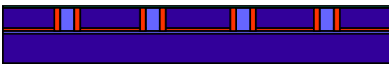
Figure 7. Cross sectional representation of the Bonded and trenched starting material. Highlighting the wrap around-region.
